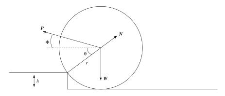
The external forces on the wheel are its weight W, the required force P acting horizontally in (a) and at an angle  $\phi$  to the horizontal in (b), and the contact forces at the kerb K and the ground G. The contact force at G may be disregarded since it disappears at the instant that the wheel starts to move. The problem is now one of static equilibrium under three forces, so the contact force at K must pass through the centre of the wheel C.
